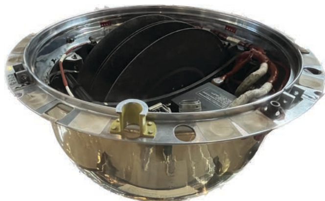
Prior to the digital age, several U.S. spy satellites used film canisters like this one to get their images back to Earth. Film was reeled into the canister and dropped from space over the ocean. A parachute would open and the canister was retrieved by a passing aircraft.
