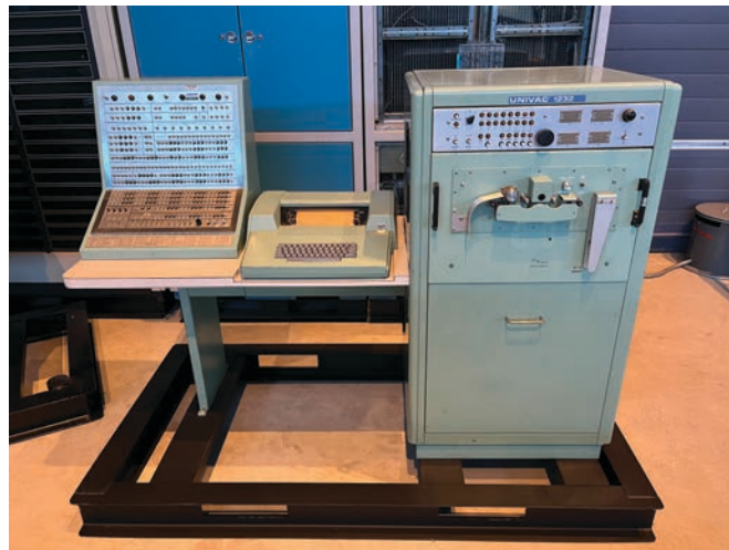
The UNIVAC 1232 computer. Used in U.S. Air Force satellite control facilities beginning in 1967, this was one of the most powerful computers available through the 1970s. It wasn't retired until 1990. It had 123 kB of memory.
