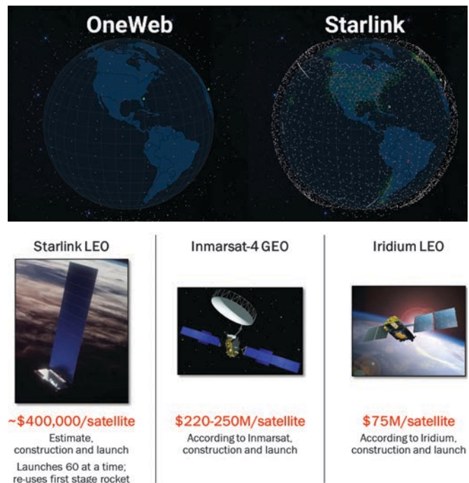
Top: StarLink's constellation of over 5000 low-earth orbit satellites compared to Eutelsat's OneWeb constellation of around 600 (and growing). OneWeb satellites are now being launched on SpaceX Falcon rockets. Bottom: Relative cost of StarLink versus other commercial satellites.
