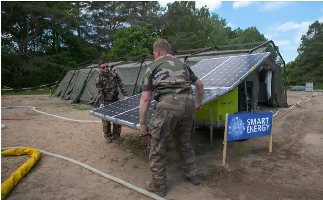
French Air Force personnel unfold a photo voltaic solar panels connected to a portable trailer that can be deployed rapidly at the NATO Smart Energy Training Assessment Camp (SETAC) which was part of Exercise CL 2019.
